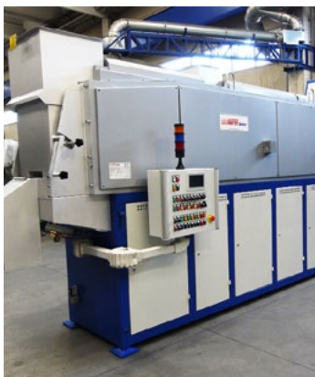
AUTOMATIC FURNACES Farm Brass furnaces (electric, gas, induction) for billet heating and heat treatment
