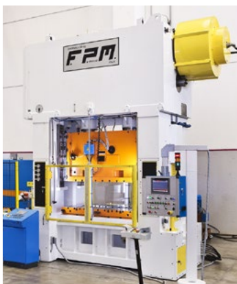
MECHANICAL PRESSES FOR COLD STAMPING of metal
